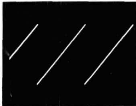
fig. 3A. Waveform from the digital sawtooth generator: three successive waves.
